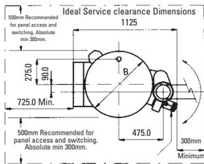
Horizontal Flue can be rotated 360°
