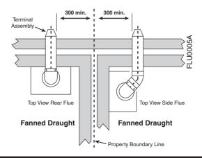
Terminal Position with Minimum Distance (mm) For IE, refer to I.S. 813 "Domestic Gas Installation".
