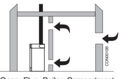
Open Flue Boiler Compartment Ventilated From Inside
