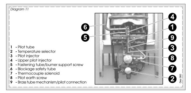
To ensure the continued efficient and safe operation of the water heater, it is recommended that it is checked and serviced annually.
