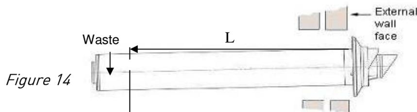
**10.13** Measuring from the back of the terminal connection, mark distance 'L' + 10mm (*figure 15*) onto the inner flue duct and cut the duct to size, ensuring that the cut is square and free from burrs.
