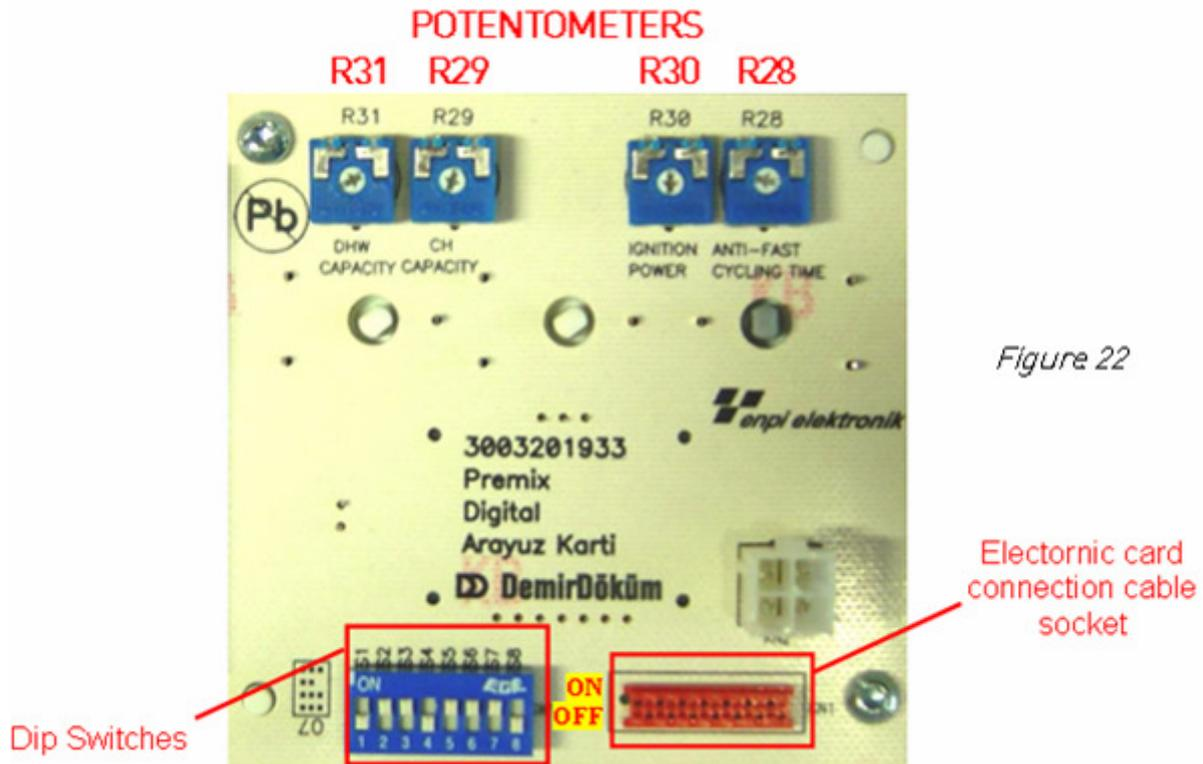
**15.2 Setting the Maximum Central Heating Flow Temperature:** The boiler is dispatched with the CH flow temperature set at 85°C. When a lower maximum temperature is required, such as in the case of under-floor heating, the factory setting can be adjusted to a maximum of 50°C giving a return temperature of 30°C, by setting dip switch 'S6' into ON position.
