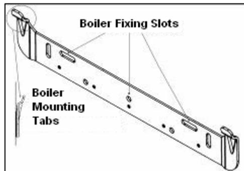
**10.6** Mount the boiler onto the fixing bracket via the boiler mounting slots, (*figure 12*).
