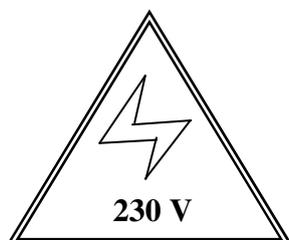
**Warning High Voltage!** This sign is located on the back of the control box housing warning of high voltages within the control box. Turn off and isolate the appliance before removing this cover.
