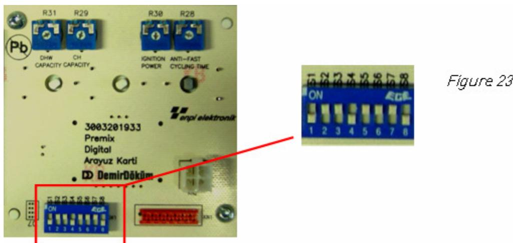
**15.5 Pump working mode setting:** The boiler has a factory set to operate the pump for pre-purge and post-purge times (45 sec.). This delay can be excluded by fitting dipswitch 'S2' (*figure 23*) into ON position. However, this may then cause the boiler over-heat thermostat to trip out.
