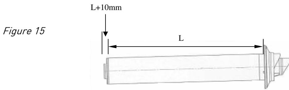
**10.14** Pass the flue assembly through the wall and connect the assembly to the boiler, ensuring that both the air and flue duct joints are fully pushed home into the connecting elbow's collar.
