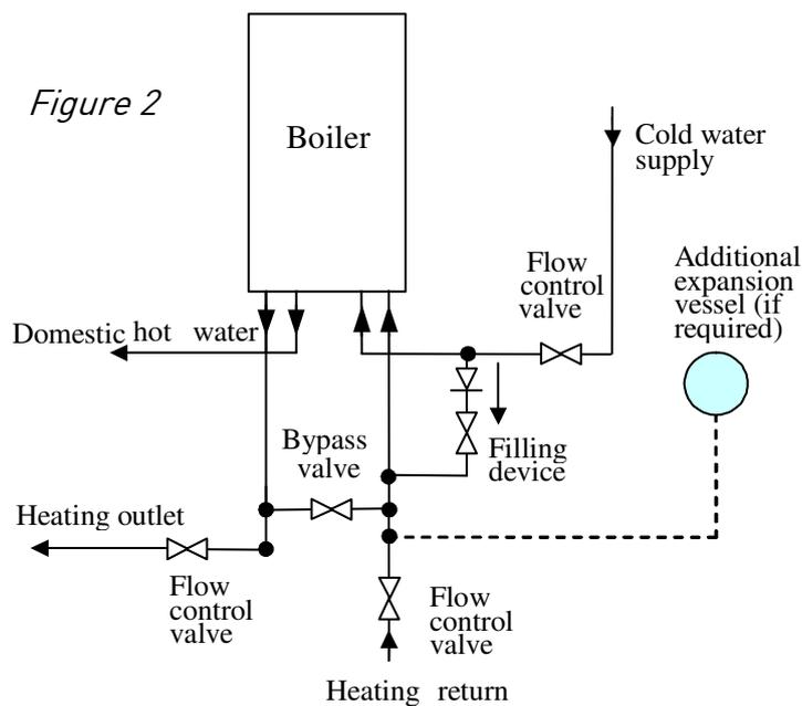
**5.4** The heating circuit should be designed and balanced to give a 20°C temperature rise across the boiler flow and return.
