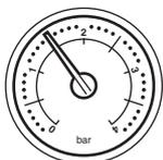
**Central Heating System Pressure** - The normal operating water pressure is between 1 and 2.0 bar. If the pressure exceeds 3 bar the safety pressure valve will operate and a fault is indicated. Contact your Installer.
