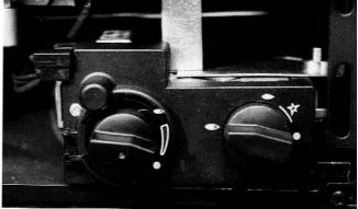
To shut the fire off completely, press the ignition control knob down and continue turning to the right from the pilot position to the OFF position.
