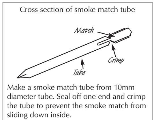
Make a smoke match tube from 10mm diameter tube. Seal off one end and crimp the tube to prevent the smoke match from sliding down inside.
