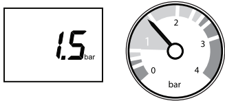
Fig.52 Restore water pressure
