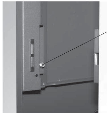
Fig. 35 Checking the setting of the door safety switch
