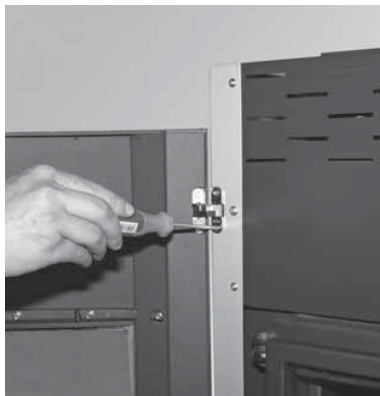
Fig. 34 Inserting the hinges in the side panel
