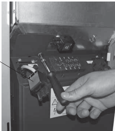
Fig. 51 Disconnecting the mains power plug and removing the screw.
