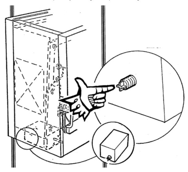
Reach into the outer case and locate the reset button at the rear of the control box. Press the button to reset the overheat thermostat.
