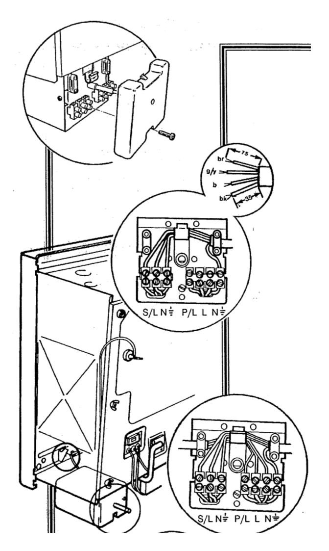
Remove the securing screw and electrical cover fastened to the thermostat box.
