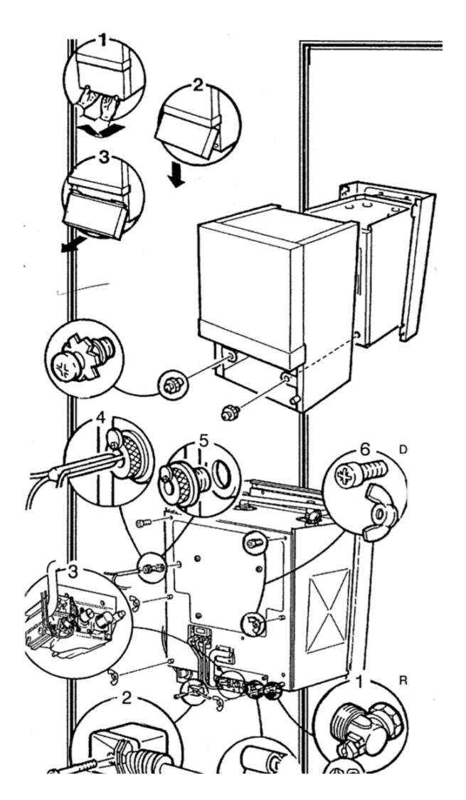
Isolate the electrical supply to the boiler.
