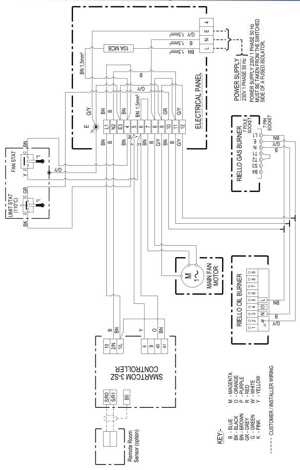
Wiring Diagram 20-45-601 60 - 85 ON/OFF Riello Burner Integral SC<sup>3</sup>-SZ 230/50/1ph
