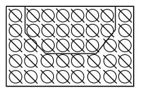
Turbulator Positions in Heat Exchanger 350 & 375 Cabinets. 28 off
