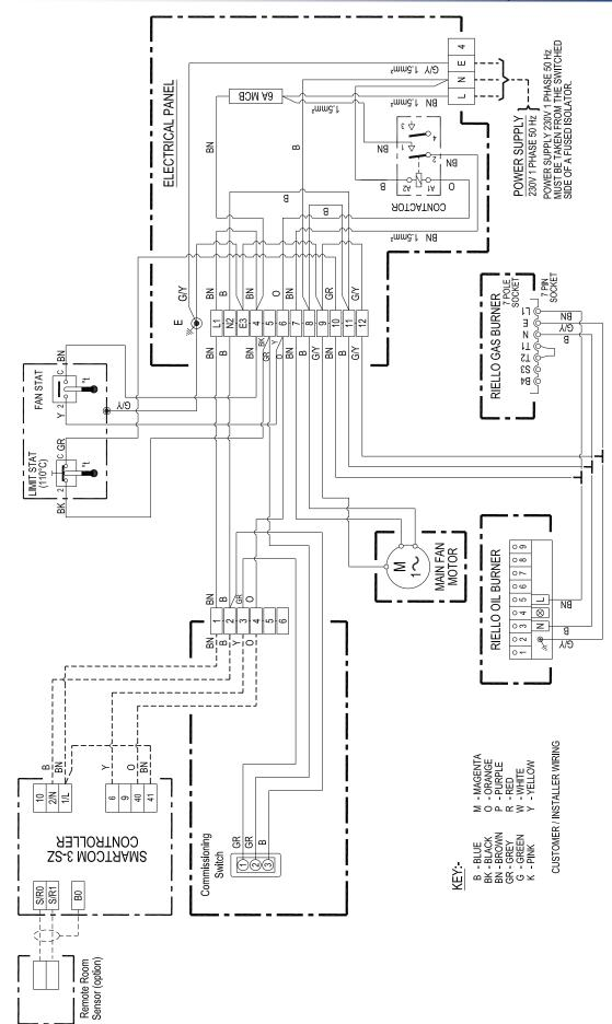
Wiring Diagram 20-45-618 120 - 135 ON/OFF Riello Burner Remote SC<sup>3</sup>-SZ 230/50/1ph
