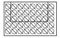
Turbulator Positions in Heat Exchanger 235 & 300 Cabinets. 40 off
