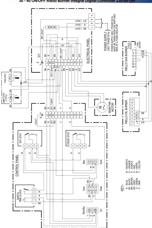
Wiring Diagram 20-45-608 30 - 40 ON/OFF Riello Burner Integral Digital Controller 230/50/1ph
