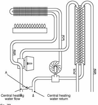
The by-pass valve is adjustable by using screw B (fig. 73); rotating it clockwise, the useful head given to the system increases.
