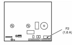
The F2 fuse can be reached by removing the service panel.
