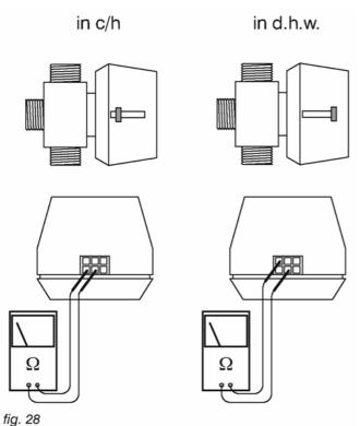
If the value is complete the resistance measured will be approx. 8  $\ensuremath{k\Omega}$
