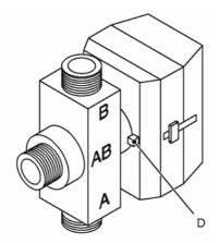
3 Release the electrical connector from the motor group.
