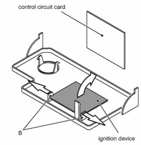
Reassemble the full sequence ignition device carrying out the removing operations in reverse order.
