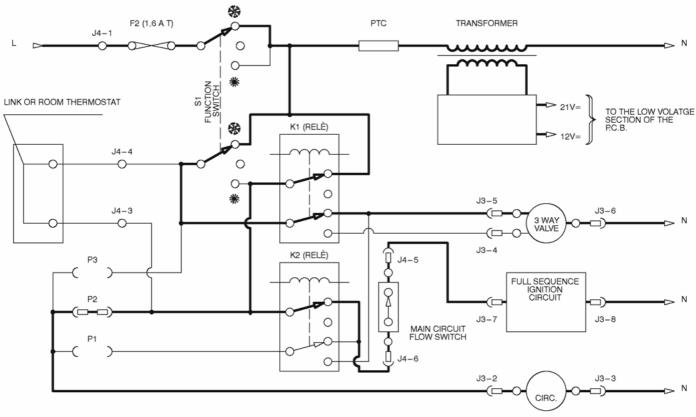
Function switch position **\*** Heat request on D.h.w.
