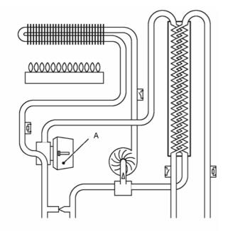
On one side of the motor body an indicator is visible with which it is possible to know the position of the diverter.
