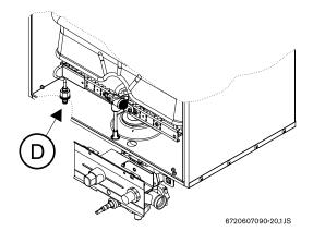
Fig. 16 - Burner pressure test point
