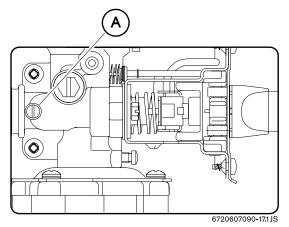
Fig. 12 - Inlet pressure test point
