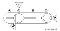
Fig. 13 - Gas control slide - Pilot ignition position
