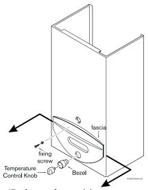
Fig. 17 - Access for servicing
