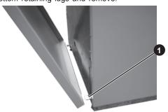
Loosen 3 screws on one side of the inner front panel and undo the 3 screws from the other side. The panel will now slide to one side for removal.
