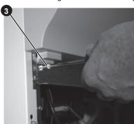
To remove completely, release the ribbon cable from the display board, raise slightly and withdraw.
