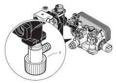
In order to drain only the water in the boiler, first shut off the heating flow and return isolating valves.
