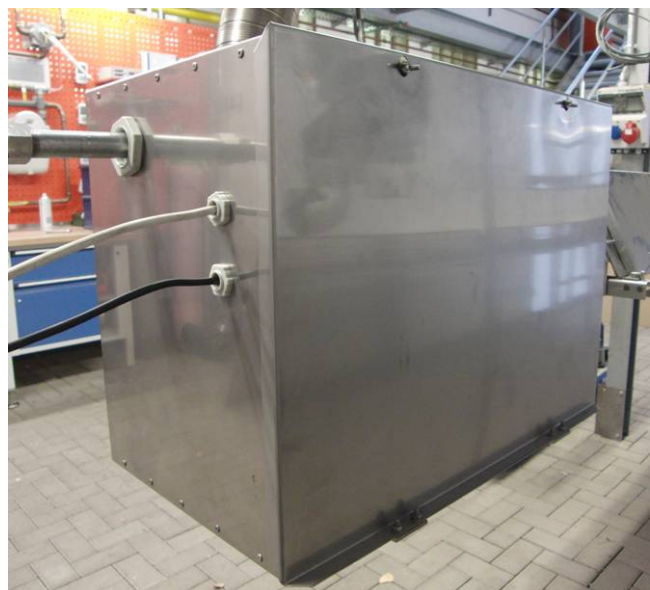
Fig. 45: Complete mounted and closed water protection cover
