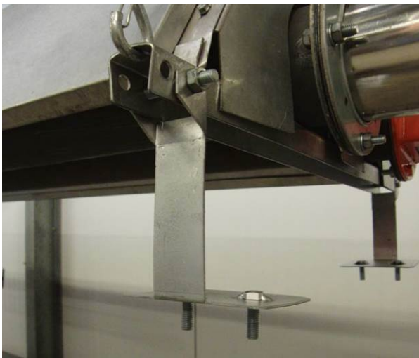
Fig. 36: Fixed angled bracket on suspension bracket
