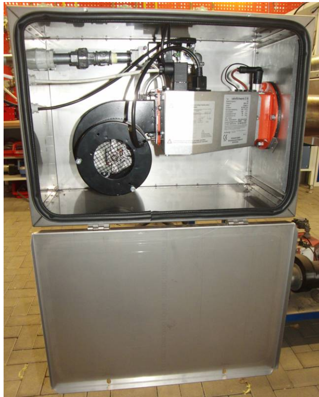
Fig. 44: Mounted burner unit in protection cover with gas inlet and electrical connections
