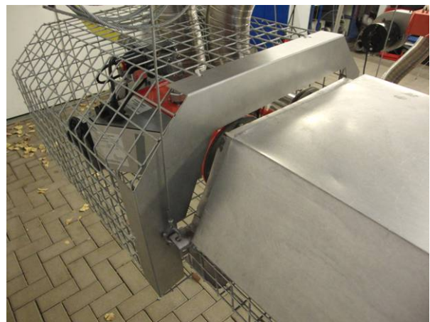
Fig. 39: Fixing front protection cover burner on protection grid burner top
